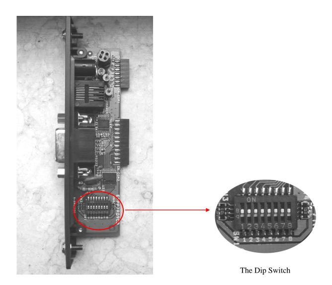
> There are 8 Dip Switch altogether, each switch has its own function, please refer to the diagram below:
